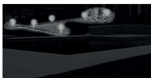
1. Uneven light, too dark on the left
