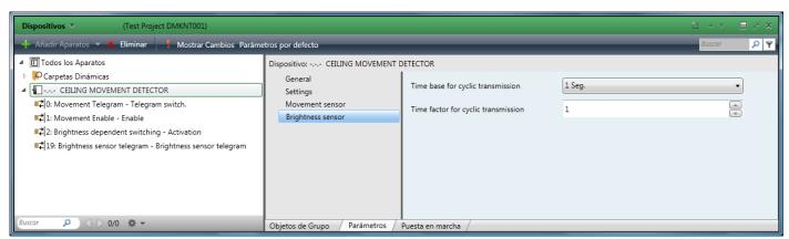
This function simply allows getting the Lux value measured by the sensor.
