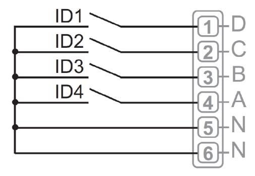
Wiring diagram as 2 analog inputs with temperature sensors (Channels C and D) and 2 binary inputs with pushbuttons or switches (Channels A and B).
