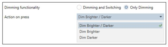
· Action on press: defines the action to be made with a short or long pressing: Dim Brighter / Darker, Dim Brighter or Dim Darker.
