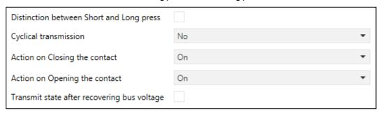
· Cyclical transmission: the object "[InX] Switch" is sent cyclically at set time intervals.
