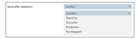
· Cyclical sending after detection: allows a cyclic sending of the corresponding value after each detection. This sending time is the result obtained from multiplying the "Time base" by the "Time factor".
