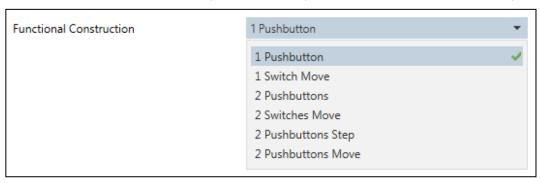
· Configuration as "I Pushbutton": sends Move Up/Down or Step telegrams, depending on the duration of the press. This function is useful when a blind must be controlled from a single button.
