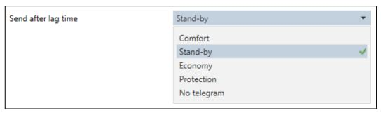
· Cyclic sending after lag time: allows a cyclic sending of the corresponding value after the delay time since the last detection. This sending time is the result obtained from multiplying the "Time base" by the "Time factor".
