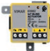
03982 Actuator for 1 roller shutter with slat orientation and change-over relay output for \cos\phi 0,6 motor 2 A 100-240 V~ 50/60 Hz, remote control, Bluetooth® wireless technology 5.0 for View Wireless mesh system and Zigbee 3.0
