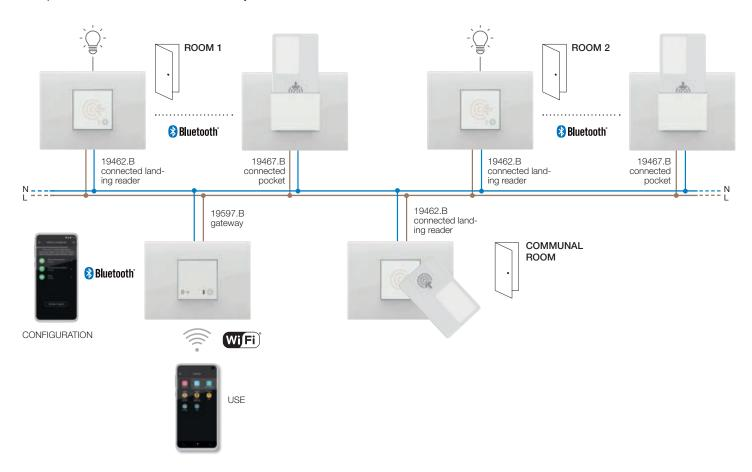
Example of the View Wireless system architecture with flush mounting devices and Zigbee technology standard:
